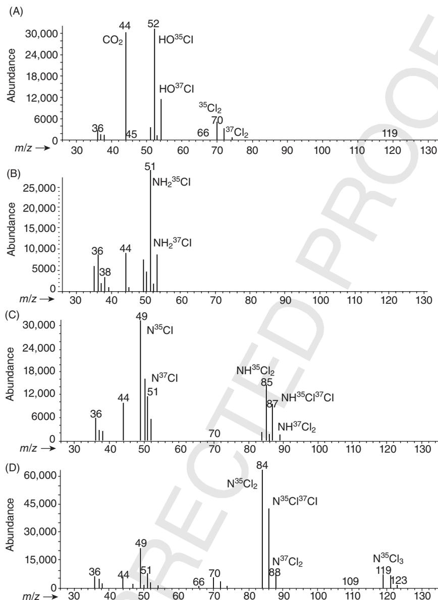
**FIGURE 27.5** Representative EI mass spectra ( $35 \leq m/z \leq 125$ ) of (A) free chlorine (2000 mg/L as Cl<sub>2</sub>), (B) monochloramine (40 mg/L as Cl<sub>2</sub>), (C) dichloramine (20 mg/L as Cl<sub>2</sub>), and (D) trichloramine (20 mg/L as Cl<sub>2</sub>). Reprinted from Shang and Blatchley [3] with the permission of the American Chemical Society.
