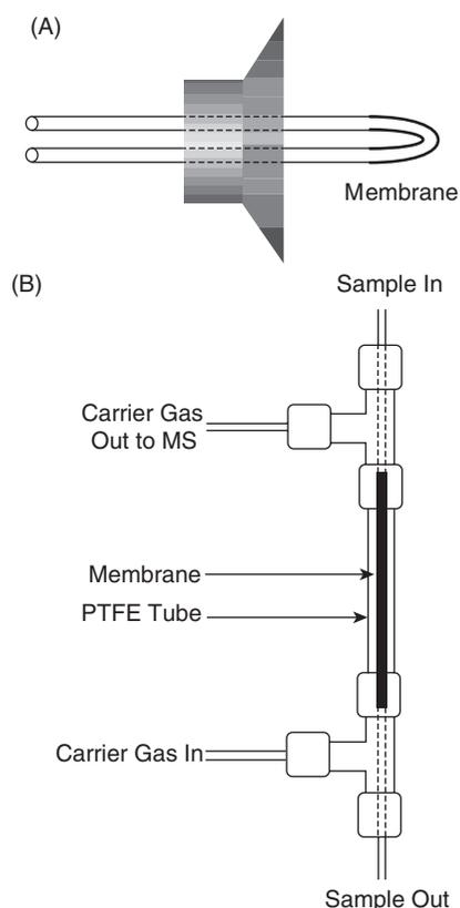
**FIGURE 27.1** Membrane introduction probes using capillary membranes. (A) A direct inlet probe and (B) an external probe. Adapted from Riter et al. [9] with the permission of the American Chemical Society.
