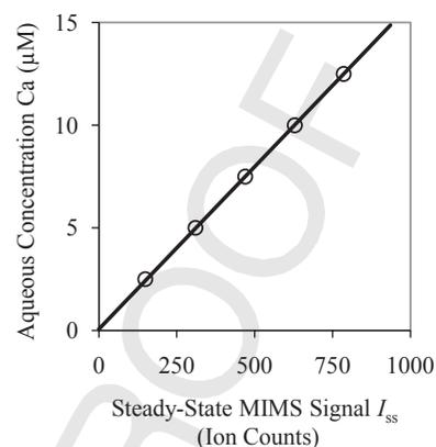
**FIGURE 27.3** A typical calibration curve for cyanogen chloride (CNCl) at pH 7.0 ( $\pm 0.1$ ) and 25°C. Experimental data are represented by gray circles, and the black line is the linear fit with Equation 27.8. Adapted from Na and Olson [17] with the permission of the American Chemical Society.
