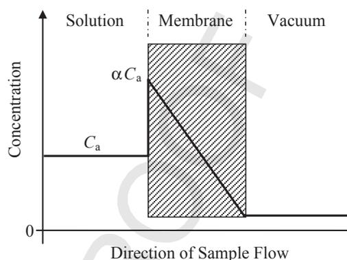
**FIGURE 27.2** Conceptual model of the pervaporation through the MIMS membrane.  $C_a$  is the analyte concentration in the aqueous solution.  $\alpha$  is the partitioning coefficient between the aqueous solution and the membrane. The linear concentration profile inside the membrane can be derived from steady-state conditions (see text for details). Adapted from Overney and Enke [15] with permission from the American Society of Mass Spectrometry.
